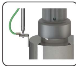
Figure 11. Ground Screw Connection
