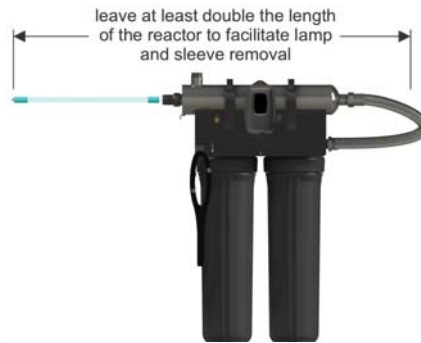
Figure 3. Lamp Removal Spacing
