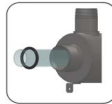
Figure 4. Quartz Sleeve Installation
