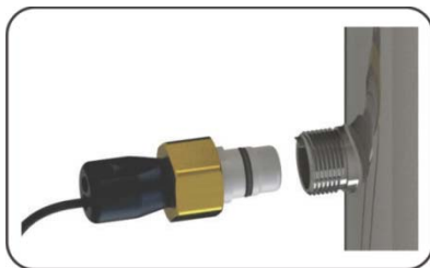
Figure 6. UV Sensor Installation
