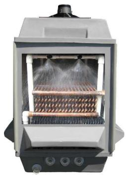
This product is a down sized version of our larger evaporative condenser line. This unit can connect up to six different refrigerated cases or A/C units, providing sub-cooling for all. Water is sprayed over the tube bundle and the fan draws air up and through the tube bundle to drive the liquid refrigerant temperature down to the mid 70 deg. F. range. The industrial design is well proven - we have similar units that have been in service for over 18 years.
