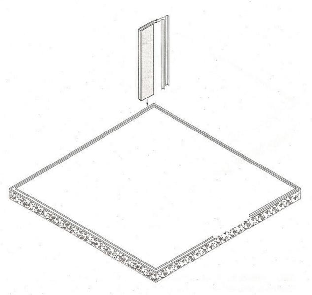
Step 2. Set one section of the panel corner unit on the base channel and install the steel angles.
