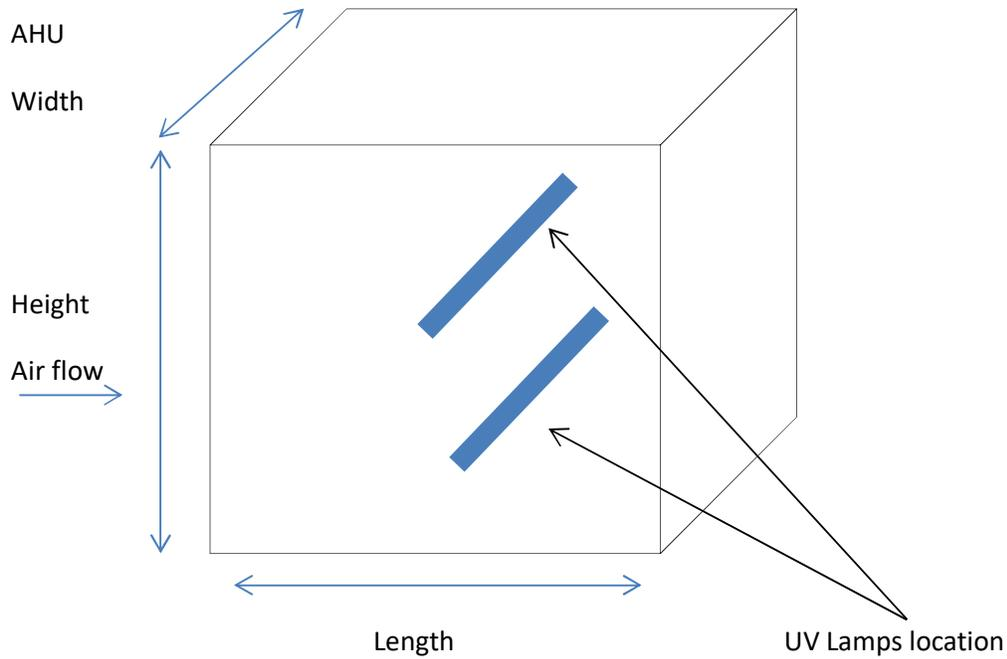
Please provide the width, height and length of the Air Handler Unit (AHU) and the CFM of air flow in order to specify the correct UV unit.
