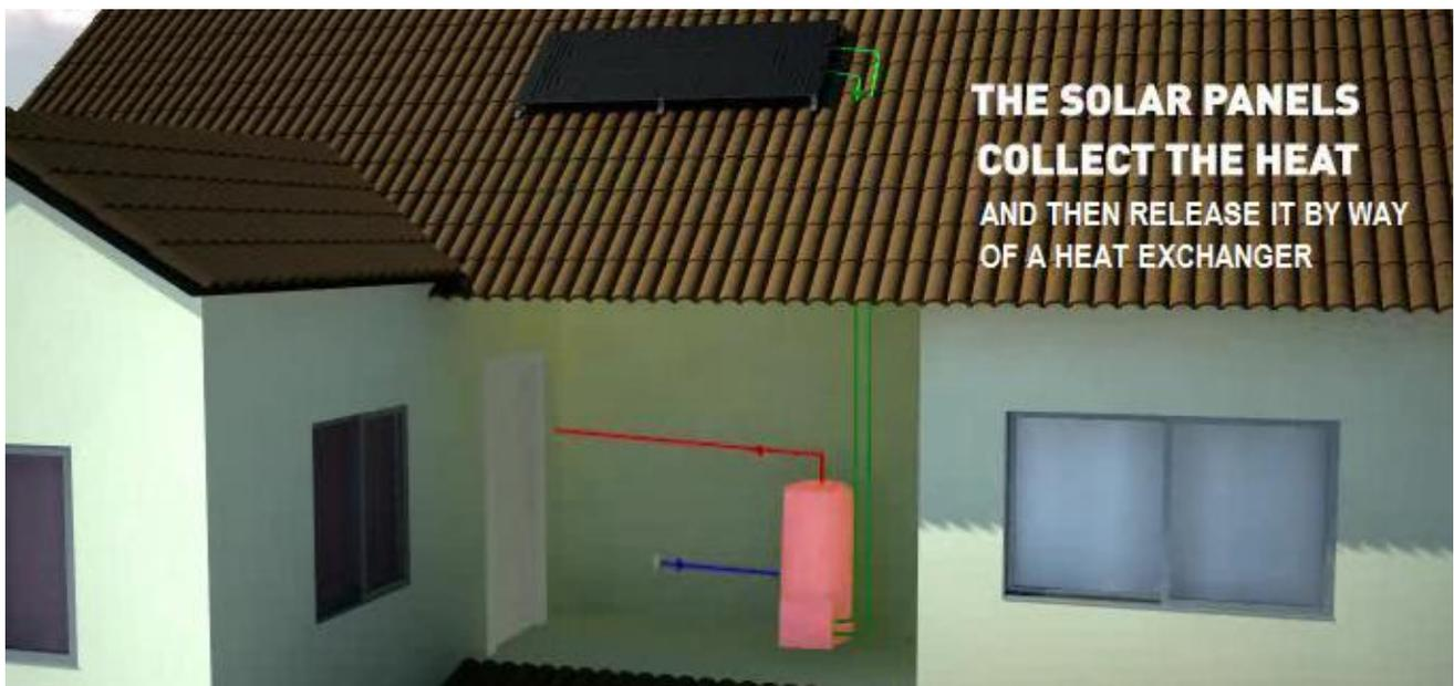
The temperature gradient caused by the external agents mentioned, ensures the **klea** (ecological cooling fluid) will evaporate inside the solar panel.
