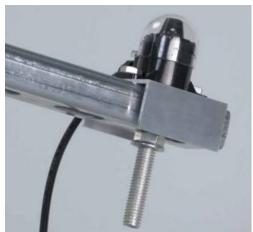
The air speed sensor needs to be put on somewhere with good ventilation, to sense the wind without any block
