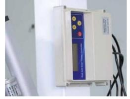
The sunshine sensor needs to be put on the mounting rod. To make it sense the sunlight when sunrise, it should be fixed on the top right corner of the brackets. There is one clamp set for putting it on, just use screwdriver to tied it
