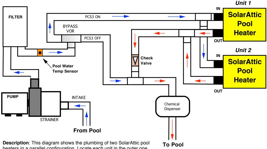
**Description**: This diagram shows the plumbing of two SolarAttic pool heaters in a parallel configuration. Locate each unit in the outer one third of the attic with the discharge pointing towards the center and at an angle to create a circular airflow pattern in the attic. Appropriate flow control plumbing valves and bypass flow circuits must also be used on large installs to optimize flow at 50 gpm through each unit.
