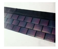
BIPV systems include shingle roofing and metal roofing with PV cells incorporated into them. These roofing systems generate electricity and provide long-lasting roofing at the same time. The amorphous silicon PV cells that are part of the roofing are guaranteed to perform to at least 80 percent of the rated power output after 20 years of use.
