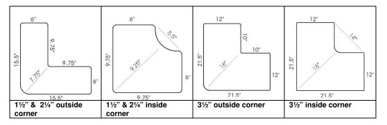
D. Wheelchair Ramps are designed to meet ADA requirements for ramp standards. Dimensions:
