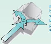
If the building envelope is breached through a broken window, wind may enter the building causing an increase in pressure that could lift the roof and push the walls outward.
