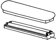
This "Cloud" fixture can be wall or ceiling mounted, with a typical use as a bathroom over-vanity fixture. A 4' fixture using two T8 lamps and an electronic ballast uses 62W of electricity to produce the light of a 95W magnetic ballast / T12 fluorescent or replaces the "Hollywood" vanity fixture with six or eight 60W incandescent globe bulbs using 360W to 480W. The core of this fixture is a fluorescent strip fixture which can be used
