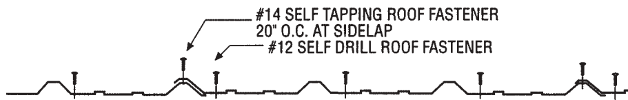
Figure #3 - Fastening Patterns for IR Panel for Wall Applications
