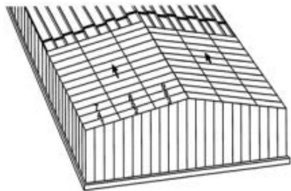
Figure #8 - Application of Sealant Tape at Side Lap
