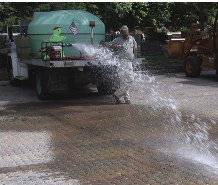
Figures 6 and 7 demonstrate permeable interlocking concrete pavement passing two important tests. The pavement passed the water infiltration test when water from the truck immediately disappeared into the surface. Just a few days prior to this test the parking lot took in a 3 in. (75 mm) rain storm with no runoff. The pavement also passed the high heel test demonstrating compatibility between fashion and environmental responsibility.
