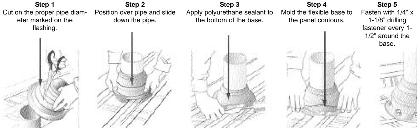
Pipe drawings provided by Triangle Fasteners
