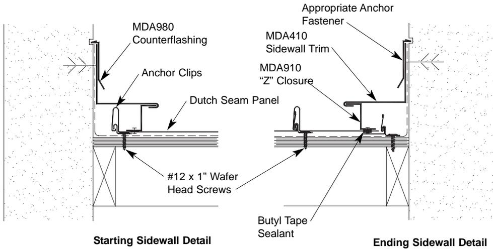
1. Install metal panel up to within 1" of the sidewall.
