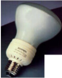
This electronic ballast compact fluorescent uses only 15W to produce the light output of a 75W incandescent lamp. The shape and size is referred to as an R-30 lamp, made for recessed cans and track lighting. The rated life of this lamp is 10,000 hours, versus 750 to 1000 hours for the incandescent equivalent. Also available in a 23W R-40 version, providing the equivalent light output of a 100W incandescent R-40 lamp.
