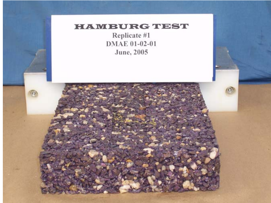
Hamburg Loaded Wheel Tester, 8,000 cycles @ 60°C – Replicate 1
